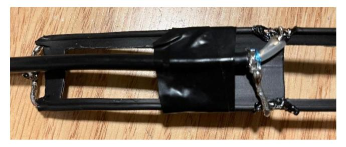
Last step before checking the tuning is to make the cut on the coax braid side.
