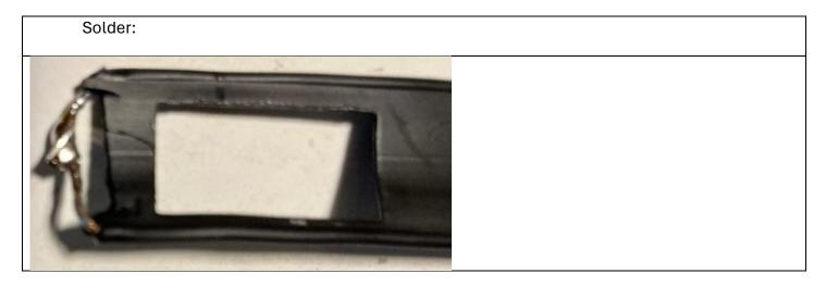
Now make the other end soldered together using the same technique - 57.5 inches away from bottom. Cut at 58 inches and strip back a half inch then solder the ends together.
