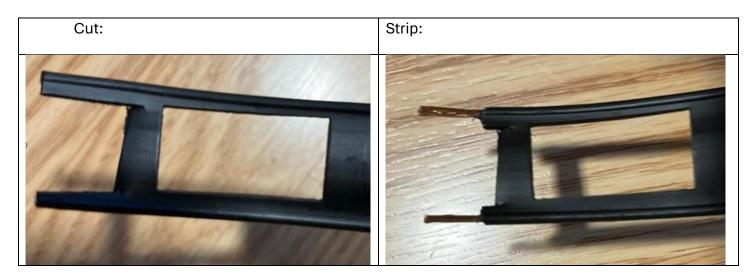
The wire is a copper-plated steel stranded wire. It's easiest to first cover the stripped wire with solder, then bend the two ends together and then solder them together. This keeps the strands together.
