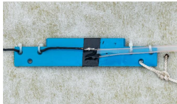
Figure 5. Transition Plate. This plastic plate provides mechanical support for the junction of the antenna wire and the 300 \Omega transmission line.
