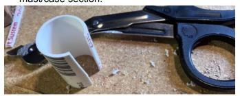
C. Depending on the intended co-ax, use a combination of inserts and tape wraps so it sits snugly in the end of the mast/case.
