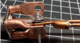
C. Rivet the assembly in place, making sure the flat washer gets caught by the deforming rivet as it starts.
