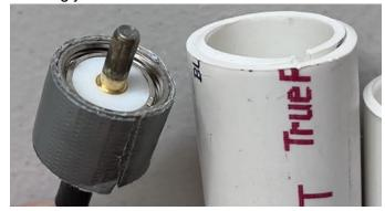
D. This tube now has an open end for stowing the antenna and a narrow end for holding it when deployed.
