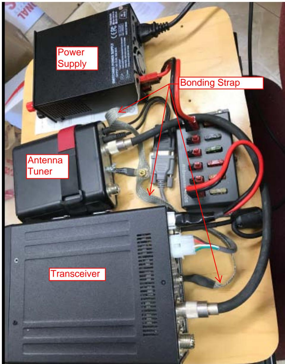
This is a close up of the bonding strap including the ground point (the brass stud and nut in the center). To complete the RF Bonding system another bonding strap would connect this point to a ground rod. Notice all the RF bonding connections are directly to the chassis of each component. Use fasteners with good conductivity. Do not use a daisy chain to connect the components. The ground point stud connects to the ground plane on the bottom of the mounting board shown in the next photo.
