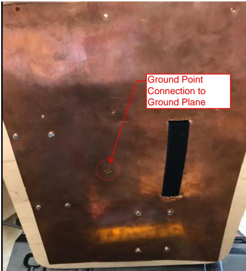
The ground plane consists of a piece of sheet copper attached to the mount board by fasteners that also attach the station components to the board. (The black strap is part of the retainer for the antenna tuner and also acts as a handle). Sheet Aluminum is also a good ground plane material. You may have to look hard to see the brass screw in the middle of the ground plane that electrically connects the ground plane to the RF bonding strap.
