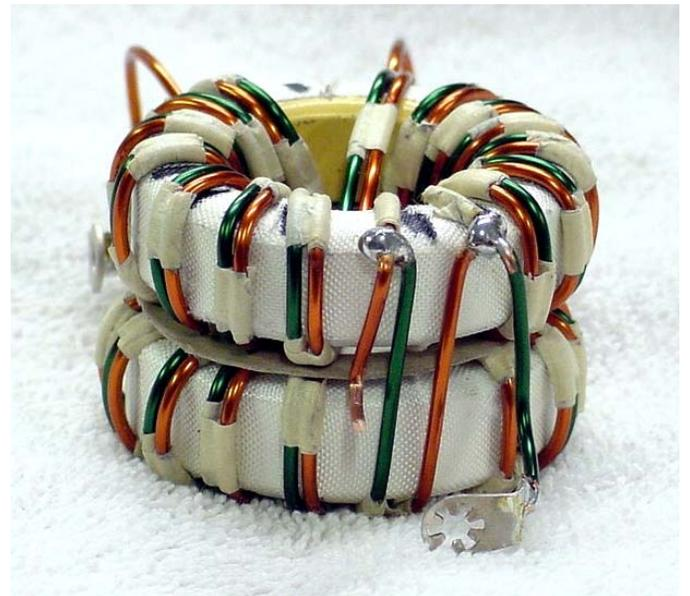
When clearance is required for scrapping insulation off a wire, gently bend/move the other wire out of the way - and remember to use smooth or rounded nose pliers. If you do not have smooth jaw pliers wrapping the tips with a few layers of tape will help to prevent nicking the insulation when forming the wires. Holding the core just above the project box will help you judge the positioning, length, and forming of the wires.
