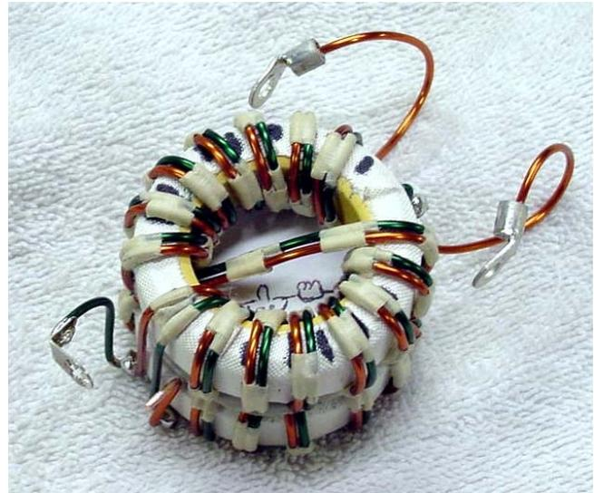
A thin cardboard spacer between the two cores will prevent damage to the magnet wire insulation. I used a separator from a 36 pack soft drink carton; cardboard from the back of a writing tablet is fine as well.
