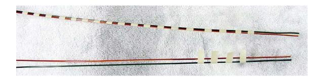
Make sure the glass tape has been applied to the outer diameter of the core before winding the transmission lines. The core coating is slippery and the glass tape adds a little *cushion* for the wire to bite into and keep the winding turns in place. I found marking the winding start and stop positions helpful. The CCW winding starts at 5 and ends at 1 o-clock, the CW winding at 7 and 11 o-clock respectively. Marking these positions help to gauge the spacing of the turns as you wind the core.
