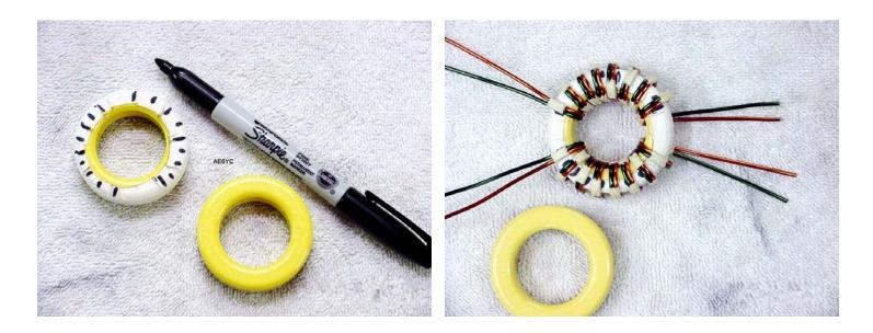
I like to start with the CCW winding. Verify the orientation of the wire colors are correct, green left, and red on the right. Start winding from the bottom of the core at the 5 o-clock location, strive for equal spacing for each of the 7 turns and end up coming off the top of the core at 1 o-clock (technically this is actually seven and a half turns).
