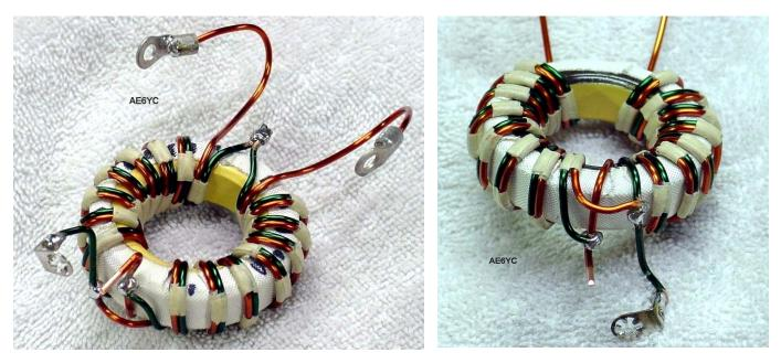
I found it easiest to start with the long green wires (# 4 and #6) near the 12 o-clock position. Cut them down to about 2 inches and scrap their insulation off. Form the wires and cut to length. Then wrap a few turns of buss wire to join the wires together, and then solder.
